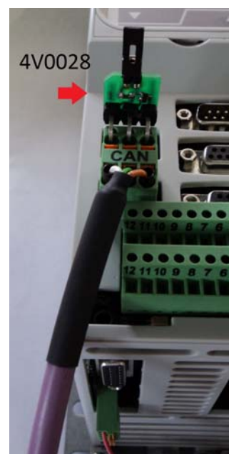
Fig. 13.1 (CAN bus termination with 4V0028)
