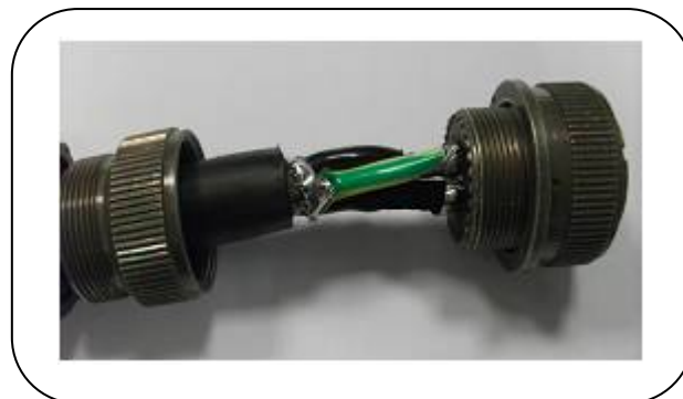
FIG. 3 (Drive side: example motor cable shield connection)
